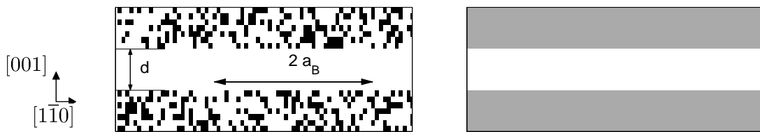
Figure 3.1: (a) Simulated cross section of a GaAs/Al 0.3 Ga 0.7 As QW ( d = 7 ML) with uncorrelated distribution of Al atoms in the Al 0.3 Ga 0.7 As layers. Al atom positions are marked in black. (b) The same structure in the virtual crystal approximation (VCA).
