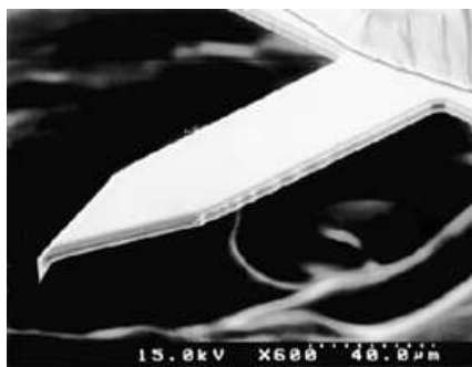
Figure 2.14: OMCL160TS Tapping TM mode cantilever, Olympus, Japan. The cantilever is 4.6 \mu\text{m} thick, 160 \mu\text{m} long, 50 \mu\text{m} wide. The height of tip is 11 \mu\text{m} and radius is less than 10 nm.
