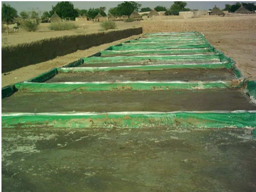
Fig 6.8: Solar energy ponds for salt drying in Elga village (Photograph by the author, Jan 2004)
