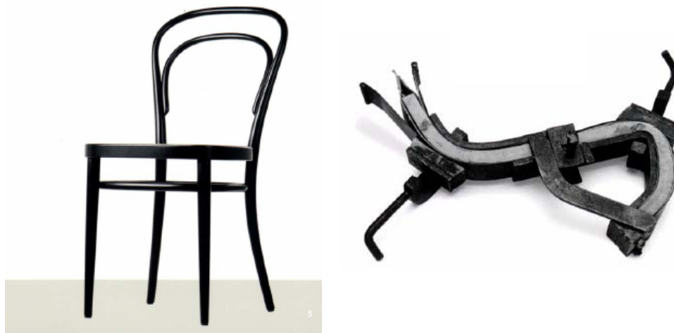
Figure 4- 9 Chair No. 14 made by Michael Thonet in 1859 (left); the mould for bending wood in Thonet (right) (ref. Thonet)
