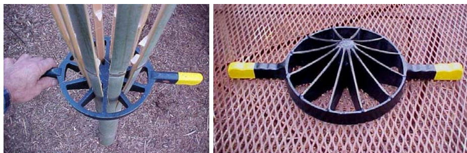
Figure 3- 4 Bamboo splitting and the tool for it (ref. Mark Meckes)
