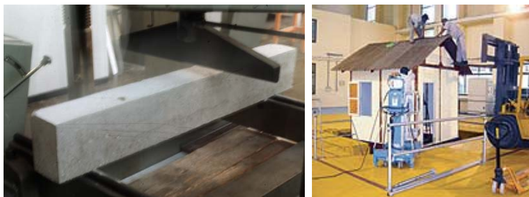
Figure 3- 18 Left: test on the bamboo reinforced concrete run by Bernd Baier in Aachen, Germany (ref. Baier); Right: house made of bamboo reinforced concrete wall and bamboo sheet roof under test at Earthquake Engineering and Vibration Research Centre in Bangalore
