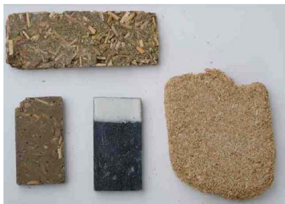
Figure 3- 16 Bamboo residual fiber can be glued together into bamboo adobe by natural glue
