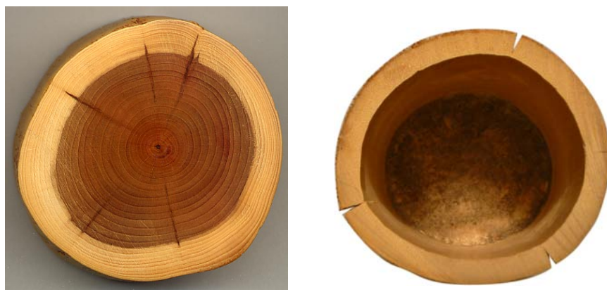
Figure 3- 23 Left: Stem section of a yew wood; right: Culm section of bamboo Phyllostachys Pubescens
