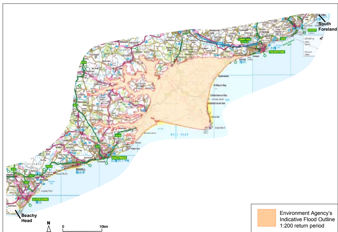
Figure 11.4 South Foreland to Beachy Head: Current coastal flooding risk
