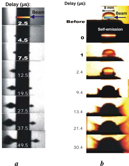
Figure 1: Superrange target dynamics in beam-target interaction experiments for 1 μs beam duration (50-200 ns exposure): (a) 6 mm thick Pb plate, Kr beam, 300 MeV/u,  $N=10^{10}$  ions, (b) 8 mm Ne crystal, U beam, 200 MeV/u,  $N=10^9$  ions
