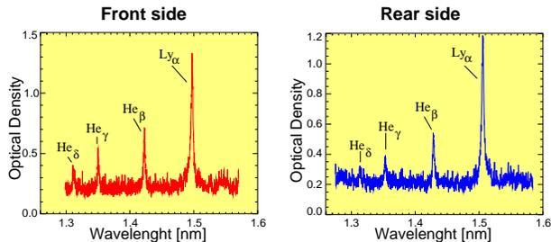
Figure 2: The comparison of X-ray spectra achieved on the front and rear surface shows similar conditions throughout the target.
