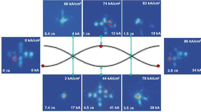
Figure 1: Image of the pepper-pot mask on the scintillator at different times during the first half wave of the current pulse
