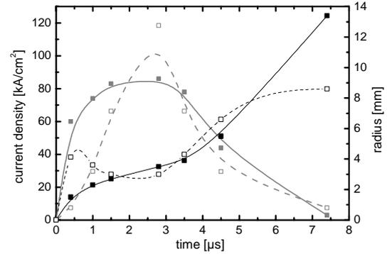
Figure 2: Development of current density and channel radius for a discharge in 17 mbar  $\text{NH}_3$ . Dashed lines are inferred from the beam transport assuming a homogeneous current distribution, solid lines from direct measurements.
