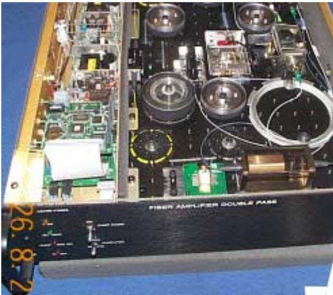
Fig. 3.: The 19" fiber-optics double-pass amplifier of the ns-frontend.
