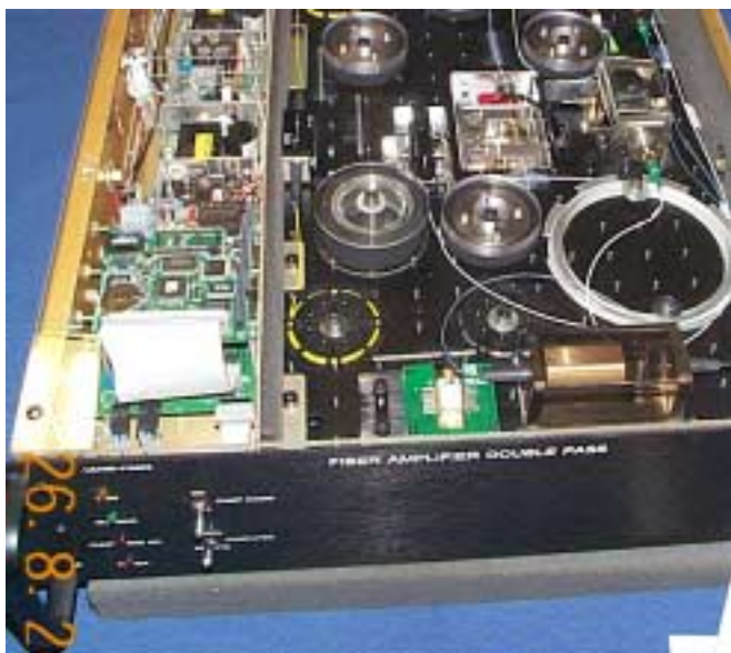
Fig. 3.: The 19" fiber-optics double-pass amplifier of the ns-frontend.
