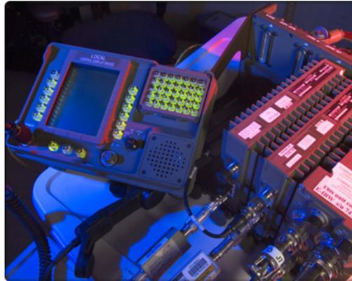
Abbildung 11.5: Joint Tactical Radio System Ground Mobile Radios
