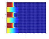
Figure 6. Retained particle concentration in a 6 layers medium with alternate filtration function  $\lambda_1 = 1 - 2\sigma m^{-1}$  and  $\lambda_2 = 20(1 - 2\sigma) m^{-1}$  after 200 days.
