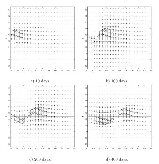
Figure 4. Vertical velocity in distinct absolute permeability layers. The horizontal and vertical axes are r and z. Particle are injected from left to right. The solid line shows the interface between the more permeable layer (top) and the less permeable one (bottom)
