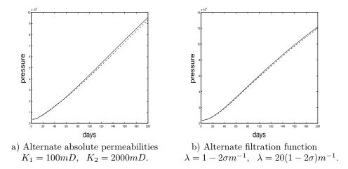
Figure 5. Pressure for communicating layers (solid line) and non communicating layers (dashed line).
