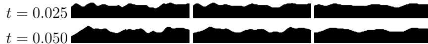
Figure 4: Film roughness in terms of correlation length l_c : Local snapshots of the film surface at times t = 0.025 and 0.05 for noise strength T = 4.05 \cdot 10^{-3} and l_c = 0, 0.5, 1 (from left to right). Discretization with a = 2^{-9} L, \tau = a^2 . For the three simulations the same sequence of random numbers have been used.
