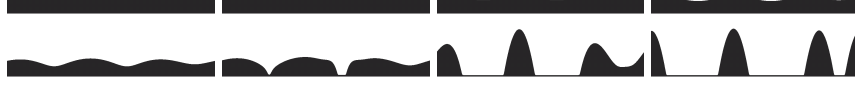
Figure 2: Snapshots at times t = 10, 12, 13, 14, 15, 15.5, 15.75, 16 for the deterministic thin-film equation. Discretisation parameters are the grid spacing a = 2^{-9} L and time step \tau = a^{\frac{5}{2}} .
