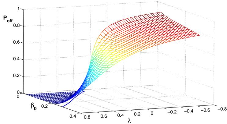
Figure 16: Separation probability  $P_{\text{off}} = \int_{-\infty}^0 dz p(z)$  according to (63) plotted over the parameter plane of contact ( $\lambda$ ) and noise ( $\beta_0$ ). In this plane the contour curve  $P_{\text{off}} = 0.05$  is drawn in blue. The other parameters are the same as in figure 15. More details are given in the text.
