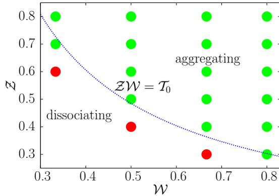
Figure 21: Tissue aggregation and dissociation depending on the relative lamella width  $\mathcal{W}$  and the dimensionless cell overlap  $\mathcal{Z}$ . The line  $\mathcal{Z} \cdot \mathcal{W} = \mathcal{T}_0 \approx 0.24 \pm 3\%$  separates associating from dissociating tissues and was determined from a linear regression against  $\mathcal{Z} = \mathcal{T}_0/\mathcal{W}$ . See also the explanations in the text.
