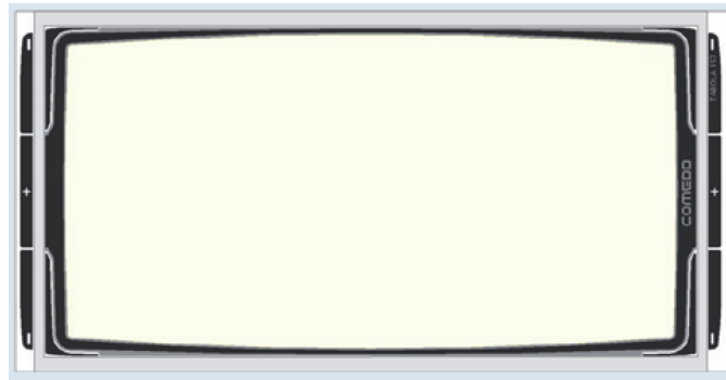
FIGURE D.13. Picture of the Tabola lighting panel used in this work with a 15\text{ cm} \times 7.5\text{ cm} large active area.
