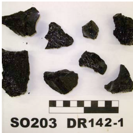
a) DR 142-1: Very fresh pieces of glass crust recovered from a volcanic cone of western axis 4A.
