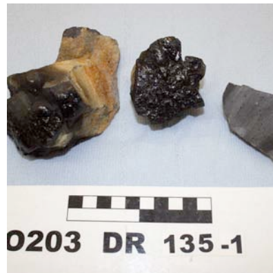
d) DR 135-1: Altered pieces of pillow lava from the eastern tip of axis 3A.
