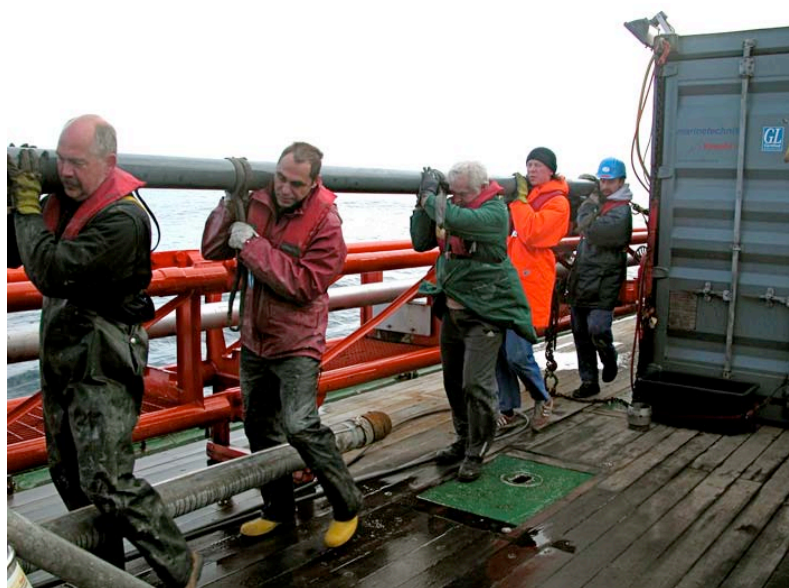
Fig. 4.11.: Successful recovery of the coreliner from the piston corer
