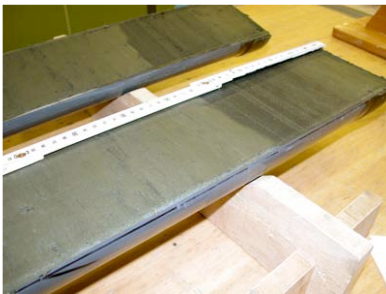
Fig. 4.4.: Core from the continental slope off Kamtchatka with turbidites.
