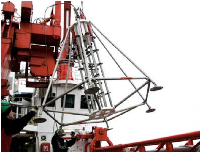
Fig. 4.5.: The „hard-ground“ Heat flow sonar system back on deck.
