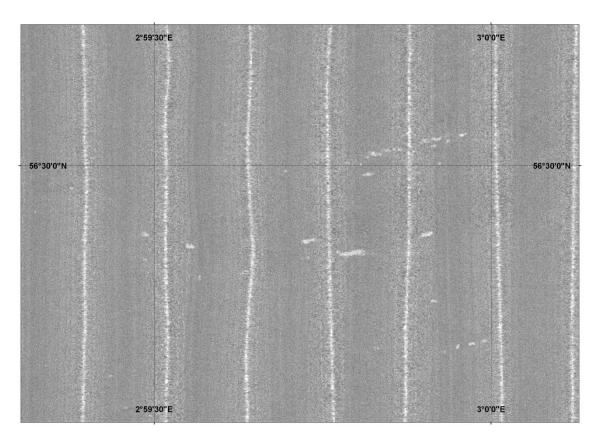
Fig. 6.2.3. Detailed map of backscatter at Tommeliten. The white dots represents a strong backscattering.
