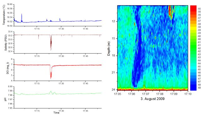
Fig. 2.3.2.3: Freshwater flare at Salt Dome Juist. Evidence from the ship CTD (left) and ADCP backscatter (right).
