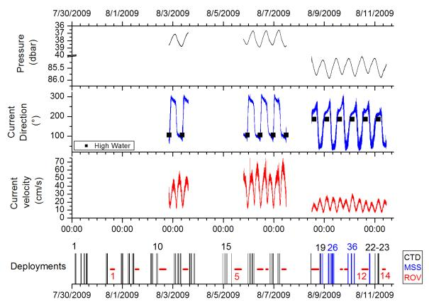
Fig. 2.1.1: Overview of the physical measurements with *in situ* recorded tidal regimes. Pressure (dbar ≈ water depth), current direction (°) and velocity (cm/s) were collected by ADCP/sensors mounted at the POZ-Lander. The bottom plot shows a timeline of the deployment for the ship CTD, the microstructure profiler (MSS CTD) and the ROV-mounted CTD with the respective cast numbers.
