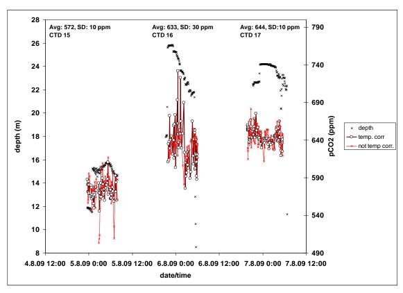
Fig. 3.3.1: pCO<sub>2</sub> recorded in the Salt Dome Juist area during 3 different towed CTD deployments (15, 16, 17) using a Membrane Inlet Mass Spectrometer. The circles represent pCO<sub>2</sub> values that were corrected for temperature fluctuations at the membrane inlet, the red lines show not corrected values. The crosses represent the depth of the CTD water sampling rosette.
