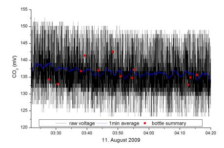
Fig. 2.4.2.2: Analog Contros HydroC/CO2 signals (CTD 23). Large noise was recorded due to malfunction of an internal pressure sensor.
