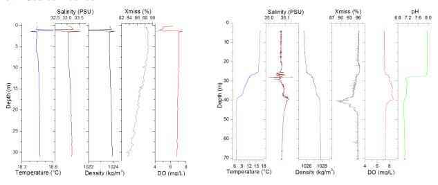
Fig. 2.3.2.2: Examples of water column characteristics from working areas (left: Borkum Riff; Right; Tommeliten).
