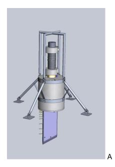
Fig. 5.1.5: Schematic drawings of the Pore Water Sampler (PWS). A: Overall setup with frame, B: Cross-section showing Rhizon lance and syringe carrier in penetration and operation modes. C: PWS with HOMER beacon deployed by ROV in the sediments sandv of the Southern German North Sea during CE0913.
