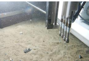
Fig. 5.2.1.1: Video-guided deployment of the Profiler Lander (PRF-L) is equipped with the microprofiler, a digital still camera system and 2 acoustic current profilers.
