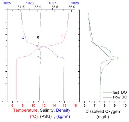
Fig. 2.5.2.2: MSS90 CTD and oxygen profiles. Left: Temperature, salinity and density profiles. Right: Oxygen profiles based on the standard oxyguard sensor (black line) and the high-resolution AMT sensor (green line).
