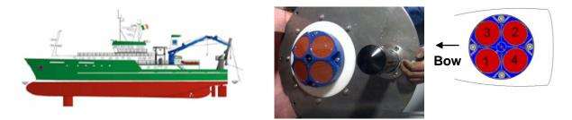
Fig. 2.2.2.1: ADCP Beam position relative to the ship and its orientation. Left: The relative position of the drop keel of the RV Celtic Explorer. Center: Mounting plate with ADCP next to the ORE Track Point transducer of the shallow water navigation system. Right: beam orientation with regards to the ship main axis.
