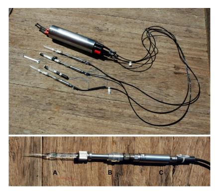
Fig. 5.2.1.2: upper panel, *in situ* micro-sensors connected to the data logging unit; lower panel, detail of *in situ* O<sub>2</sub> microsensor (A) connected to the amplifier (C) via an oil filled steel tube (B).
