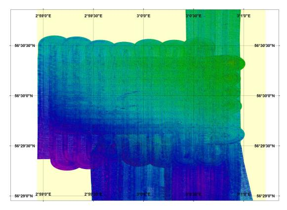
Fig. 6.2.1: Bathymetry map of Tommeliten. The blue spots represent small depressions, around 40 cm compared to the surrounding area.
