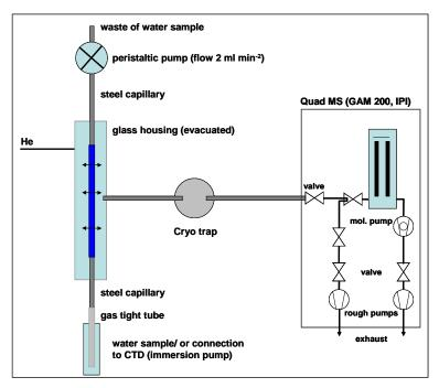
Fig. 3.2.2: Scheme of the set up of the Membrane Inlet Mass Spectrometer. For details see text.
