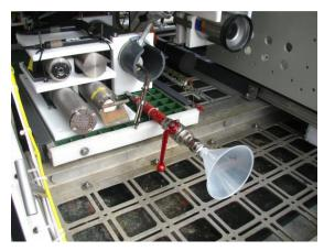
Fig. 5.1.4: View of starboard drawer with CONTROS probes, gas sampler, KIPS nozzle and HDTV camera.
