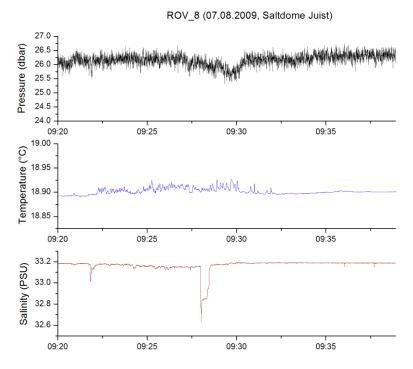
Fig. 2.3.3.1: Salinity drops at the Saltdome Juist site, as seen on the ship CTD and ADCP (Figure 2.3.2.3).
