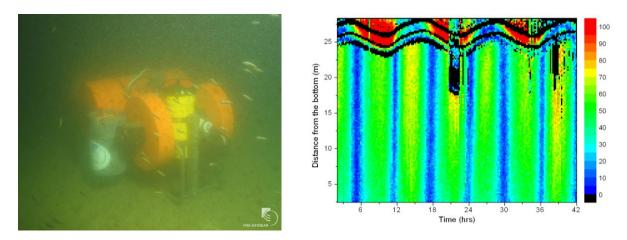
Fig. 2.2.3.1: Left: POZ-lander with Workhorse ADCP. Right: Current velocity magnitude (cm/s) as well as the tidal driven water level changes as record by the ADCP on the POZ-Lander at the Saltdome Juist site. Note that the black spots are due to the ship cruising over the POZ-Lander location.
