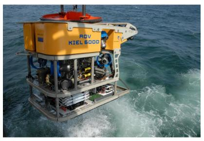
Fig. 5.1.1: Views of ROV Kiel 6000; left: front with cameras, manipulators and tool sled for storage of the push corers; right: starbord side with KIPS water sampler, CONTROS sensor package and FSI CTD.
