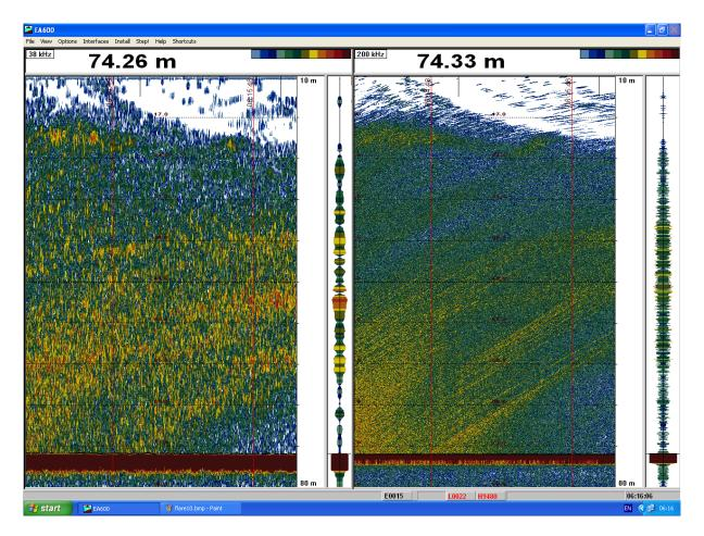
Fig. 6.2.5: Gas flare at Tommeliten covering the whole water column.
