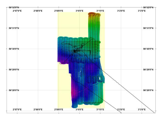
Fig. 6.1.2. Bathymetric map from Tommeliten. The difference between the shallow area (red colour) and the deep area (purple colour) is around 3 meters.
