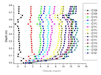
Fig. 2.2.4.1: Left: Profiler lander showing positions of the RDI ADCP (top white circle) and the Nortek High-Resolution ADP (bottom circle). Right: Current profile time series in the BBL with a 30-mm spatial resolution. Bottom is estimated slightly to be a few mm below 0.0. The profiles show the temporal evolution (starting with the black) of the increasing current direction with a 15-minute resolution. Developed flow field follow law-of-the-wall velocity distribution.
