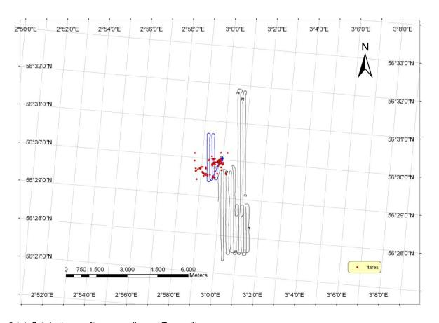
Fig. 6.1.1: Sub-bottom profiler survey lines at Tommeliten.
