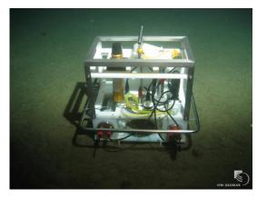
Fig. 5.1.7: Benthic Chamber (BC) equipped with syringe water sampler, oxygen optodes, stirrer, power and control unit, and HOMER beacon deployed at Tommeliten.
