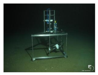
Fig. 5.1.9: One of two Eddy Correlation Systems (ECS) deployed by ROV at Tommeliten (for detailed description see chapter 5.3).
