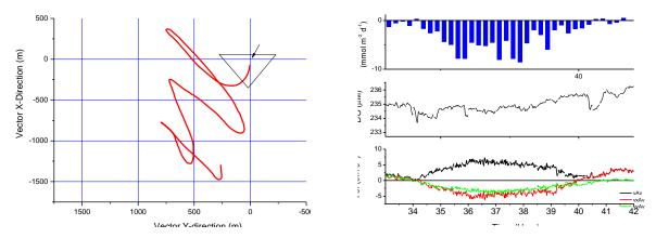
Fig. 5.3.2.1: Eddy Correlation Technique. Graphical visualization of the path, with respect to the EC device, of a single water parcel moved around by the current over the whole deployment time (left); preliminary results from one of our system (right), velocity components (bottom), DO concentration (center) and the calculated DO fluxes into the sediment (top).
