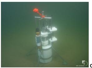
The Benthic Chambers (BC) are designed to measure benthic fluxes of dissolved chemical species over time at the sediment-water interface. They contain a cylindrical chamber (20 cm diameter)
