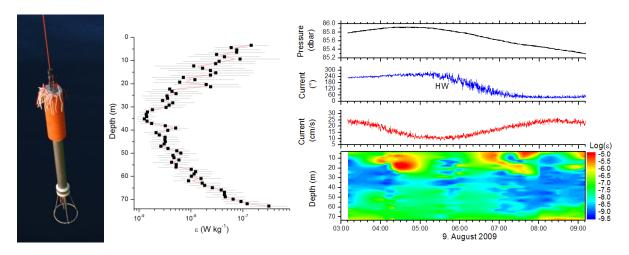
Fig. 2.5.2.1: MSS Probe and results overview. Left: the MSS90 profiler being retrieved. Center: Averaged turbulence level profile calculated from the shear probe sensor readings. Right: turbulence level contour plot (bottom) with the consequent tidal information from the POZ-Lander (see Section 2.1.1).
