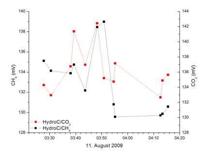
Fig. 2.4.2.1: Analog Contros HydroC recorded at the same time of the fired Niskin-bottles at the Tommeliten site (CTD 23).
