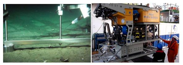
Fig. 5.3.1.1: Eddy Correlation (EC) Technique. Our EC system on the North Sea bottom (left) and on the ROV Kiel 6000 during the pre-deployment.
