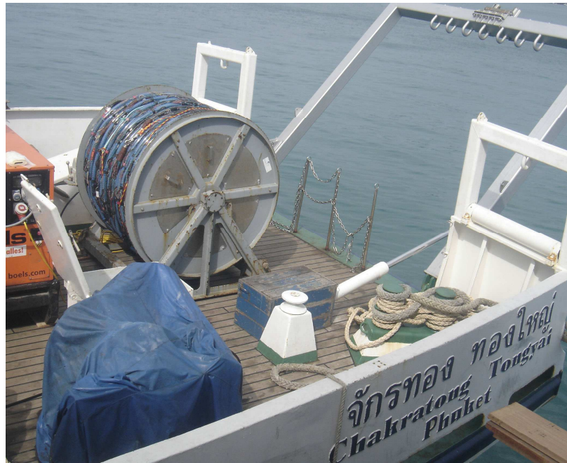
Fig. 12: Picture of the streamer system (on the winch) which was used on RV Chakratong Tongyai during the MASS III-cruise.
