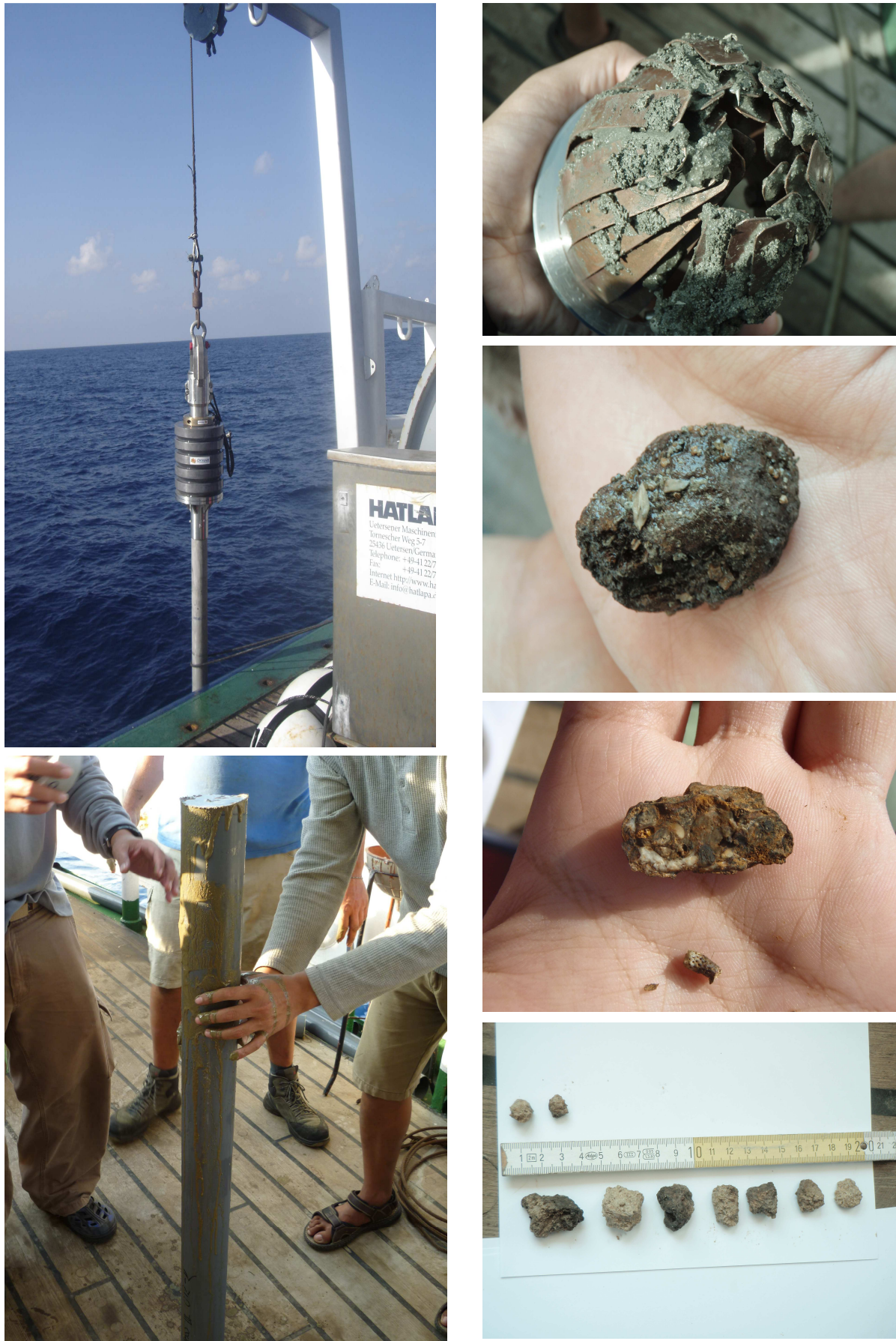
Fig. 21: Mini-Gravity Corer launched at the stern of Chakratong Tongyai. Recovered sediment core and seafloor material received from the core catcher.
