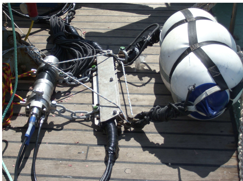
Fig. 11: Micro GI-Gun (0.11) used during seismic surveying on Chakratong Tongyai.
