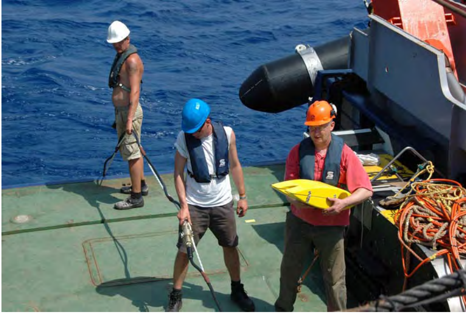
Figure 5.2.2.4: Floats are fixed on the cross cable in order to keep it at about 2 m depth during profiling
