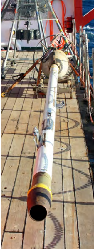
Figure 5.5.1.1: Views of the gravity corer.
