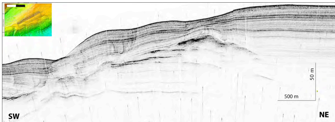
Figure 6.1.3.1: An example of 4 KHz Parasound data beneath Opouawe Bank, looking towards the NNW. Data are plotted at a 10x vertical exaggeration. Vertical streaks in this image (as well as in Figure 4) are noise bursts that have not been removed for this particular image.
