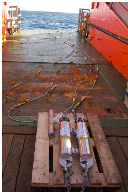
Figure 5.8.1: Sketch of the mooring layout (left) and parts of the mooring (releasers and thermistor string) laying on the back deck of SONNE during assembling.
