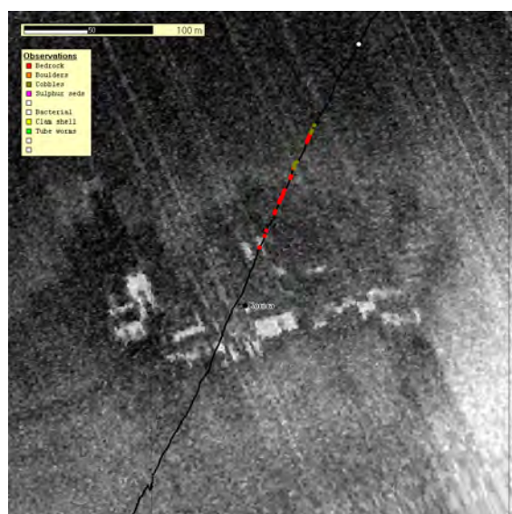
Figure 6.6.1.7: Korora site, OFOS-5. No seep-related substrates or fauna were observed at this site. Note, the geo-referencing of either the sidescan sonar image or the OFOS track is evidently incorrect because the high-relief substrate indicated by strong backscatter in the sonar image should coincide with the observations of bedrock outcrops from the OFOS video.
