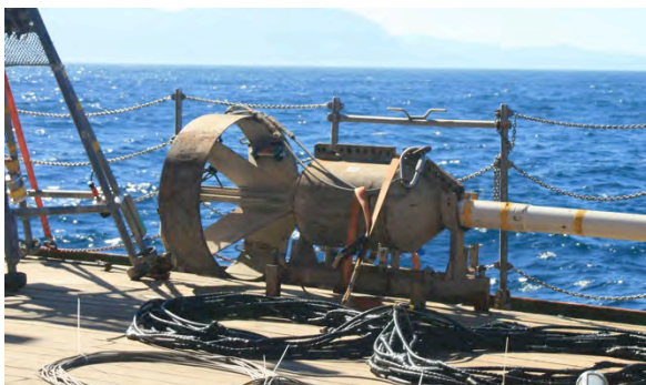
Figure 5.5.1.1.a Photograph of the lead filled weight with fins
