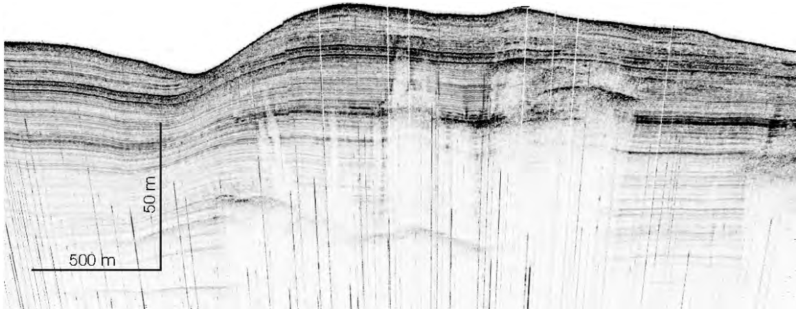
Figure 6.1.3.2: An example of 4 KHz Parasound data beneath Opouawe Bank, looking towards the SSE. Data are plotted at a 10x vertical exaggeration.
