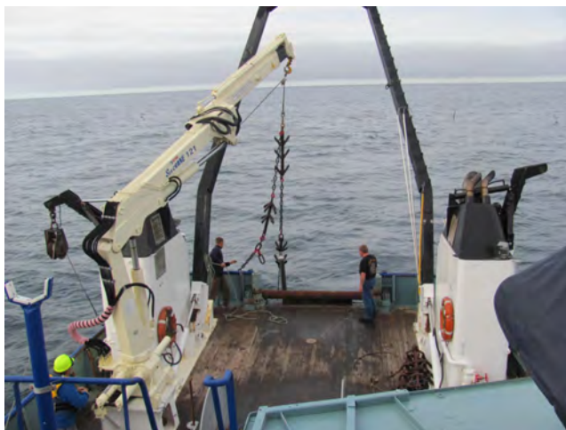
Figure 6.4.1.10: Instrument recovery on NIWA vessel RV Kaharoa. After nine attempts the last receiver was finally picked up by the hook. All four receiver units and the data were recovered.
