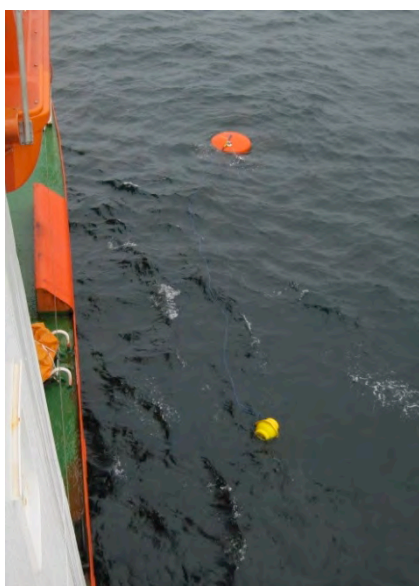
Figure 5.8.3: Mooring drifting by the vessel and being recovered.
