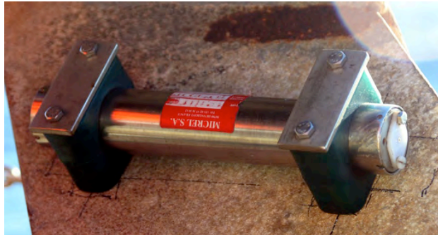
Figure 5.5.1.3. The tilt meter mounted to the fin of the bomb.
