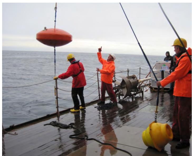
Figure 5.8.3: Mooring drifting by the vessel and being recovered.
