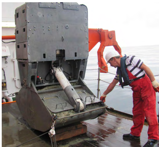
Figure 6.4.1.8: left: OFOS with recovery hook, top: TV Grab, bottom: Cable tension on TV Grab while pulling up. Increase and sudden release in tension suggests, the array slipped off the grab at 690m cable length (about 370m above seafloor).
