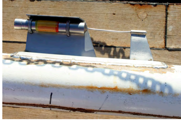
Figure 5.5.1.2. One of the 5 temperature sensors, attached to the core barrel.
