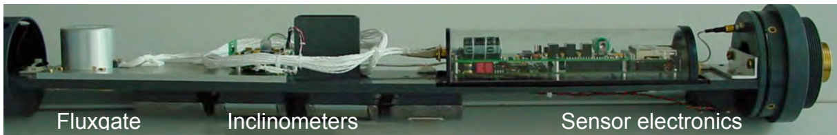
Fig. 6.2.: Components inside the fluxgate magnetometer towfish.
