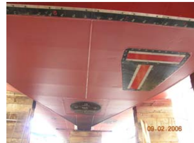
Figure 6.6.4: transmitting and receiving transducer of the EM710
