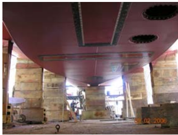
Figure 6.6.2: METEOR's hull below waterline, construction holding the transmitting (front) and receiving transducer of the EM120
