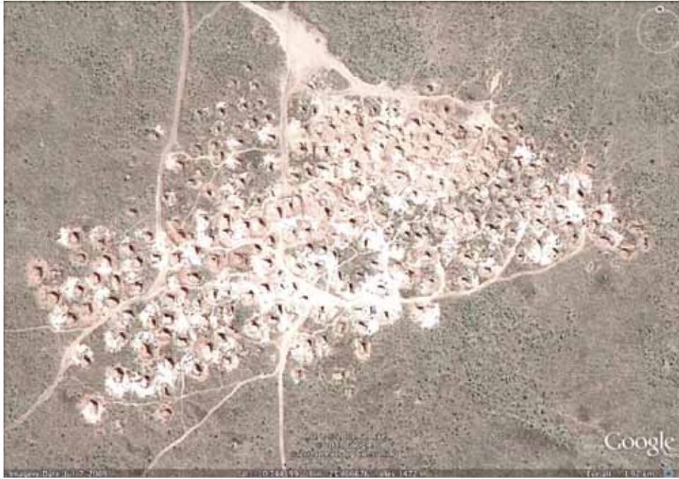
Figure 3. Satellite image of artisanal mining near Kolwezi in the DRC. The per-area damage impact on land cover of the actual digging is obviously very high; however, areas of such intense artisanal digging are uncommon. The dimensions of this digging site are about 500 m × 250 m.
