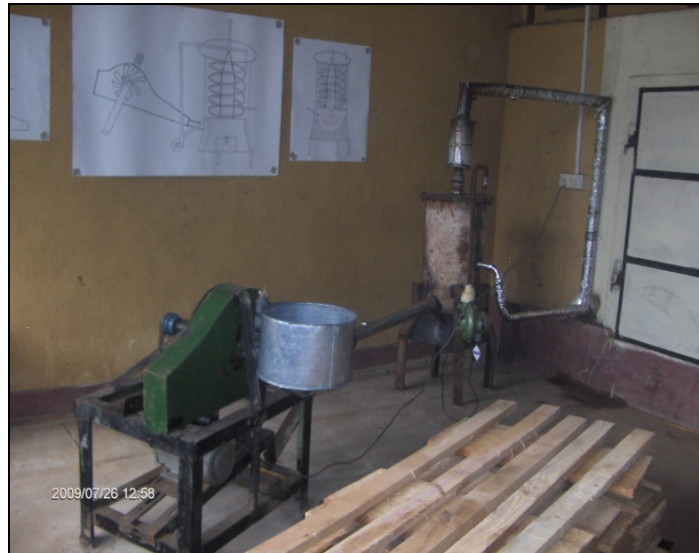
Figure 2. Prototype sawdust burner at the university premises
