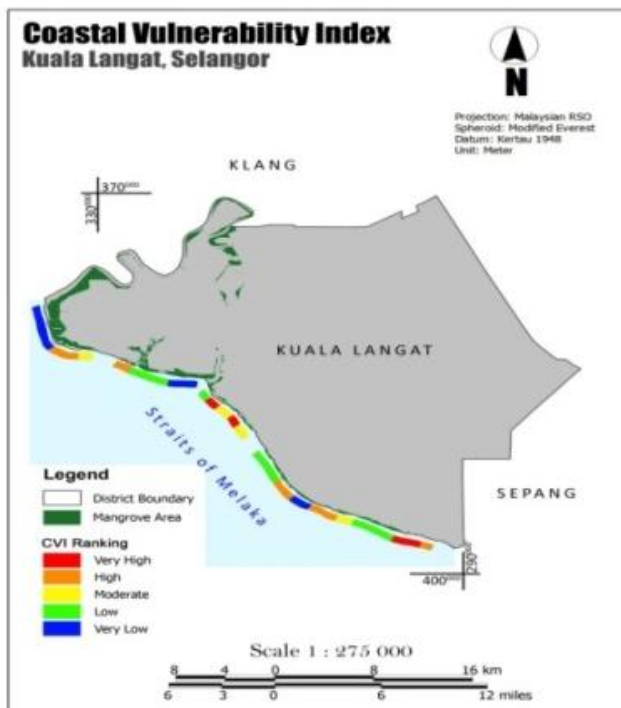
Figure 1. Coastal Vulnerability Index to future sea level rise for the coast of Kuala Langat.
