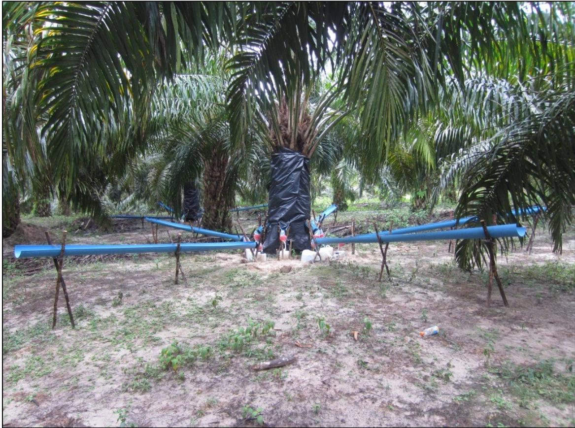
**Fig. 6.** On-going research includes measurement of water interception by oil palms. Photograph by Suria Tarigan.
