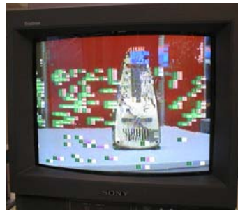
Fig.4: Severe Blocking in Areas with Strong Movements
