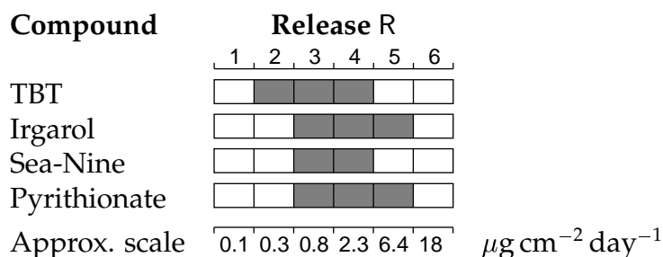
Figure 6.1: Indicator values of the four biocides selected for the release rate evaluation. The bar charts show the range of the indicator values, where 1 means the lowest release and 6 means the highest release necessary for fouling control in combination with copper
