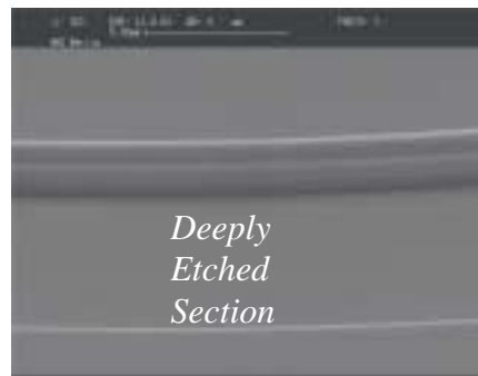
Fig. 60: SEM – photograph of an asymmetric waveguide in the curvature.
