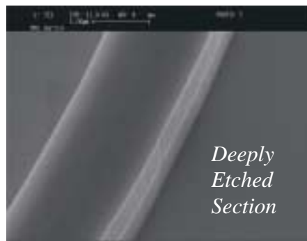
Fig. 61: SEM – photograph of the deeply etched curvature.
