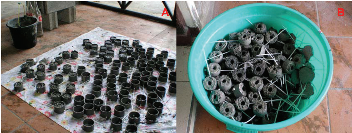
Figure 2.4: Bases for the coral transplants were manufactured from concrete (A). The finished bases included a hole for fitting the coral transplants (B).
